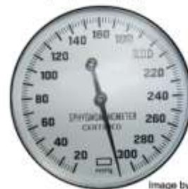
Pressure gauge of a sphygmomanometer
